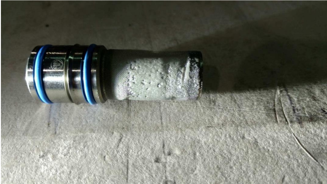
Figure 2: DEF crystallization on aircraft fuel filter.
