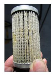
Figure 2. DEF crystals in fuel filter. PHOTO COURTESY OF FAA
